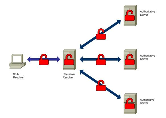
The recursive resolver is in a privileged position to log all of the DNS queries and responses. After all, DNS queries are explicitly sent to the recursive resolver by the stub resolvers.
